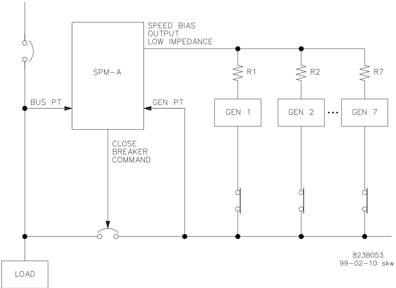
Figure 3-2. Synchronizing Bus to Bus
